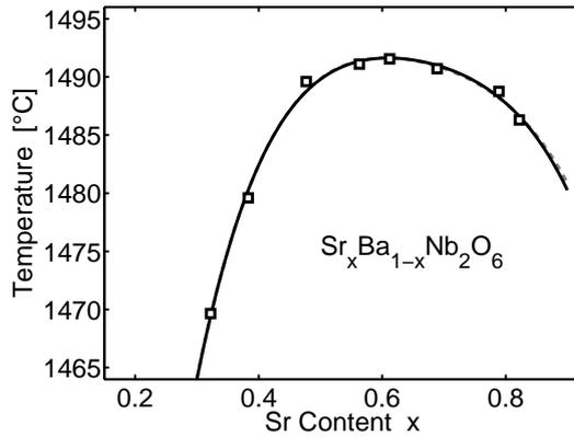
Figure 3: Solidus curve of Strontium Barium Niobate. The dots denote the measured values, the black solid curve is a fourth order polynomial fit to the data with the maximum forced to  $x = 0.61$ . The gray dashed curve again represents the unconstrained fit, the difference, however, is hardly detectable.
