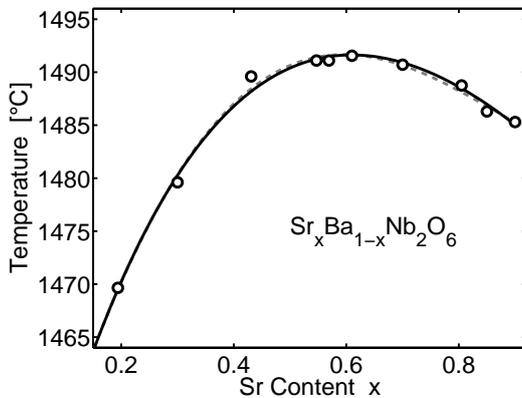
Figure 2: Liquidus curve of Strontium Barium Niobate. The dots denote the measured values, the gray dashed curve is an unconstrained fourth order polynomial fit to the data, the black solid curve is a fit with the maximum forced to  $x = 0.61$ .
