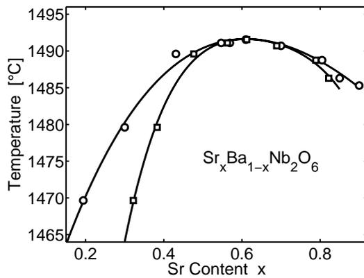
Figure 4: Phase diagram of Strontium Barium Niobate. The dots denote the measured values for the liquidus and the solidus compositions and temperatures, the black curves are fourth order polynomial fits to the data with the maximum forced to  $x = 0.61$ .
