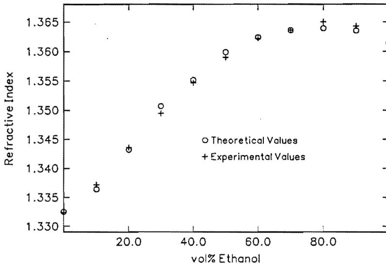
FIGURE 3: Refractive indices measured(+) and calculated(o) for water-ethanol mixtures. The parabolic dependence is due to the volume changes.
