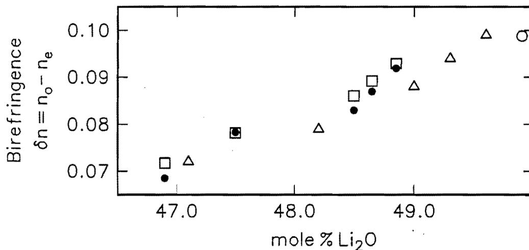
FIGURE 5: Birefringence of LiNbO<sub>3</sub> as a function of the Li content ( $\lambda = 632.8$  nm,  $T = 17$  °C). •: difference of the refractive index values from fig. 4, □: Hofmann<sup>8</sup>, Δ: Carruthers et al.<sup>9</sup>, ○: Jundt et al.<sup>10</sup>.
