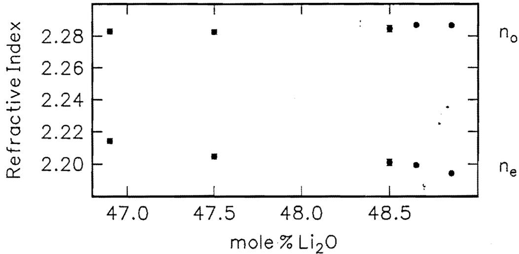
FIGURE 4: Ordinary ( $n_o$ ) and extraordinary ( $n_e$ ) refractive index of LiNbO<sub>3</sub> as a function of the Li content ( $\lambda = 632.8$  nm,  $T = 17$  °C).
