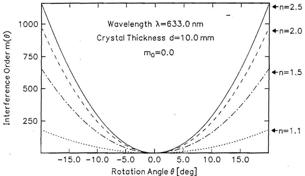
FIGURE 1: Fringe shift function  $m(\theta)$  for various refractive indices.
